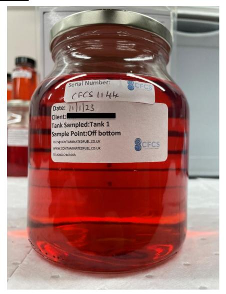
Clear and bright to ASTM D4176, no free water, no debris, no MBG, moisture content <200PPM, ISO 4406 19/17/12, flashpoint >55, FAME 0.08%, cetane 49.3, density 827, ATP Test 0 RLU's, DCI 50.72, cloudpoint -11.1, FBT 1.02, Viscosity @40c 2.2.
