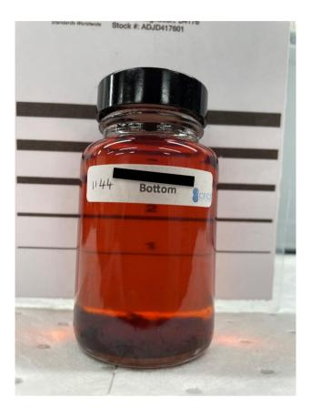
The sample has minimal evidence of free water in the formation of droplets and some debris and MBG.
